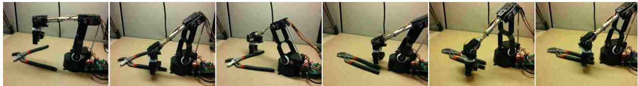
Figure 5.4: The robot makes mistakes but fixes them. Sequence of images from left to right shows the performance of the robot. The task here is to close and orient the water pump pliers. When the pliers are pushed more than expected, the robot turns around and pushes the other side to move the pliers back to the desired orientation.
